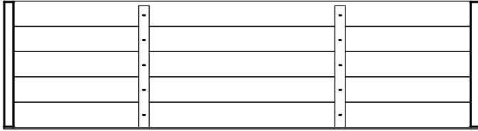
(1) RP3 - ROOF PANEL - W2A01862 1 3/8"x16 1/8"x59 1/2" (35x410x1532)
